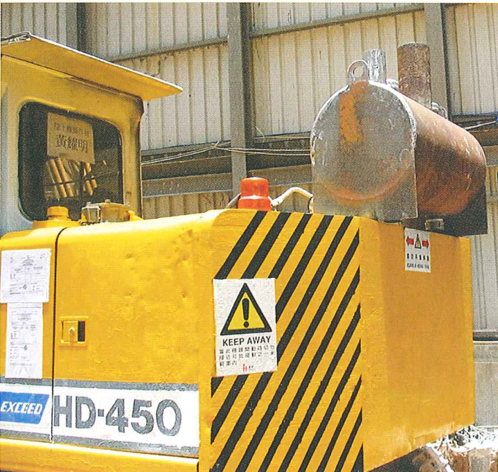
Water scrubber mounted on a backhoe to mitigate exhaust fume 在挖泥機上裝置水性隔氣鼓以減少在操作挖泥機時所產生之廢氣
